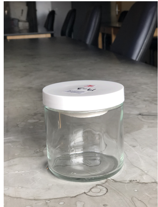
Figure 1-9: An ethyl acetate-charged kill jar for dispatching insects that are caught alive.
